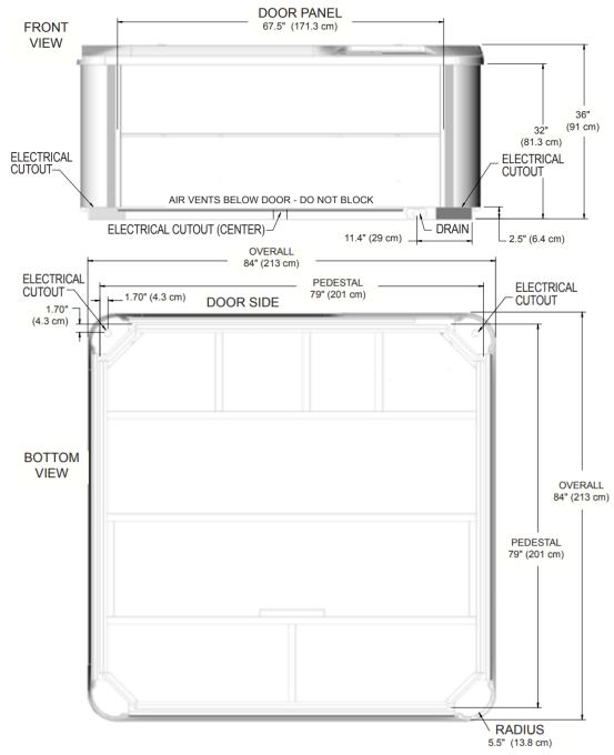
**NOTE:** Watkins Wellness recommends that your tub be installed on a minimum 4" (10 cm) thick reinforced concrete pad or structurally sound deck that is able to support the "dead weight" found in the spa specification chart on pages 6 and 7.
