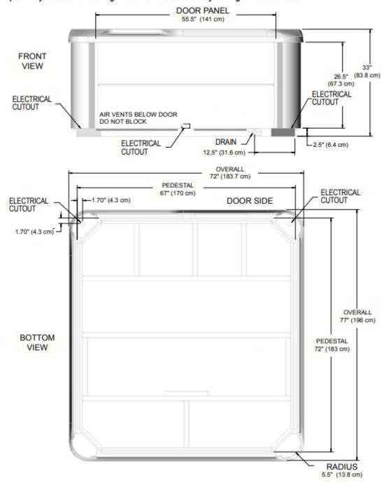
**NOTE:** Watkins Wellness recommends that the SX be installed on a minimum 4" (10 cm) thick reinforced concrete pad or structurally sound deck that is able to support the "dead weight" found in the spa specification chart.
