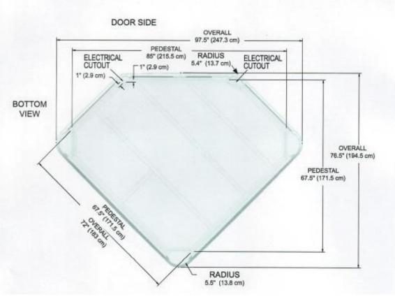
**NOTE:** Watkins Wellness recommends that the TX be installed on a minimum 4" (10 cm) thick reinforced concrete pad or structurally sound deck that is able to support the "dead weight" found in the spa specification chart.
