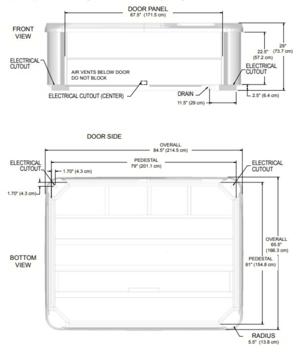
**NOTE:** Watkins Wellness recommends that the STRIDE be installed on a minimum 4" (10 cm) thick reinforced concrete pad or structurally sound deck that is able to support the "dead weight" found in the spa specification chart.
