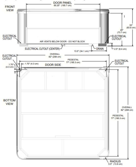
**NOTE:** Watkins Wellness recommends that the PACE be installed on a minimum 4" (10 cm) thick reinforced concrete pad or structurally sound deck that is able to support the "dead weight" found in the spa specification chart.
