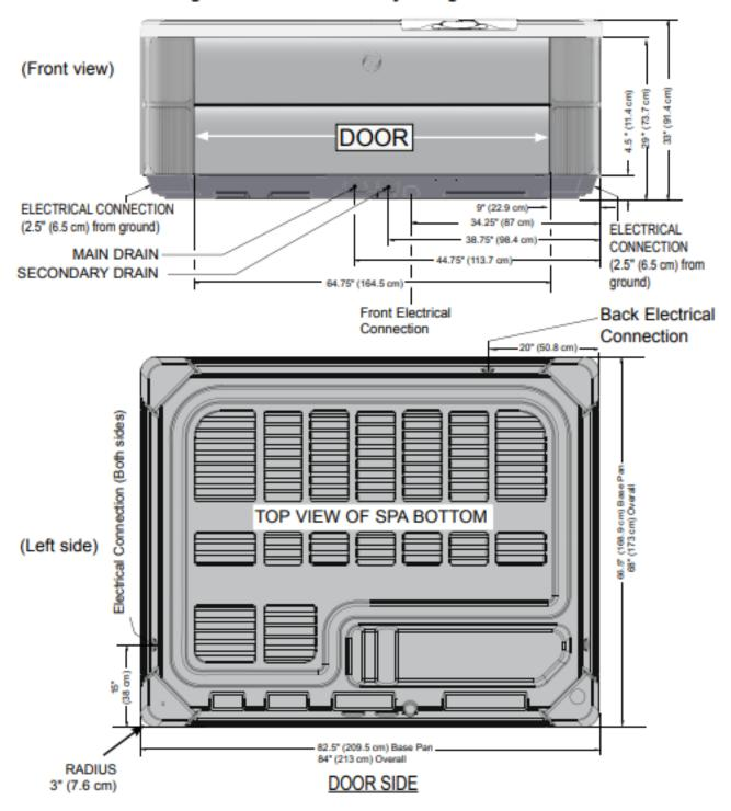
NOTE: WATKINS WELLNESS recommends that the JETSETTER be installed on a minimum 4" (10 cm) thick reinforced concrete pad or a deck that is able to withstand more than 115 lbs/ft<sup>2</sup> (555 kg/m<sup>2</sup>).
