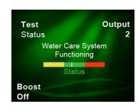
Displays Output Setting Press Soft key to scroll through settings.
