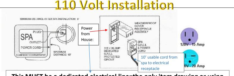
This MUST be a dedicated electrical line=the only item drawing or using electrical power on this line. ANY shared line will not run the hot tub!
